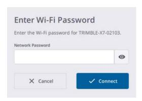
7. If you forgot the password you can reset the password to the factory default value by pressing the On/Off button on the instrument for twenty seconds. You will hear beep, followed by three consecutive beeps after ten seconds and then five consecutive beeps after ten more seconds. Release the On/Off button to complete the reset. Perspective will prompt you to set the password again the next time you try to connect to the instrument.
